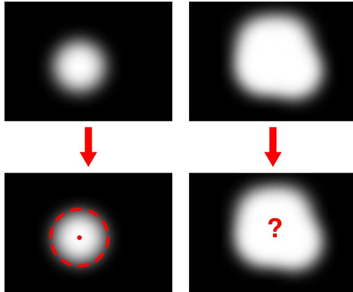
(a) For a single emitter, its position can be determined rather accurately from its diffraction-limited image.
