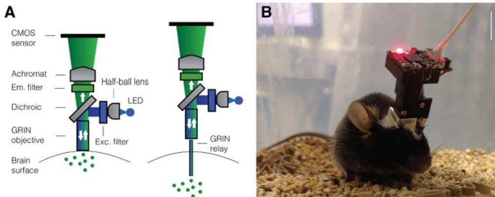
Figure 5: A. A typical design of a miniscope. Notice the GRIN lenses that allow both to deliver the excitation light to the brain and to collect the emitted light. The miniscope on the left is used for imaging the surface of the brain, while the thinner GRIN relay lens of the miniscope on the right can be inserted deep into brain tissue. B. A mouse carrying a 3-g UCLA miniscope. Scale bar, 10 mm. Image from Aharoni and Hoogland (2019).
