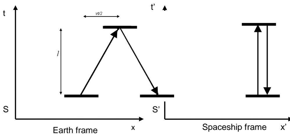
If the above diagram is not obvious, think about the simultaneity of events discussed in the links above. We can call the light pulse leaving and arriving at mirrors “events”: points in both space and time. In  $S'$  the light pulse hits a mirror and is reflected back. If the mirror and pulse weren't at the same point at the same time the pulse would just keep going as it was. Whichever frame we are in, all observers have to agree that the light pulse hits the mirror.
