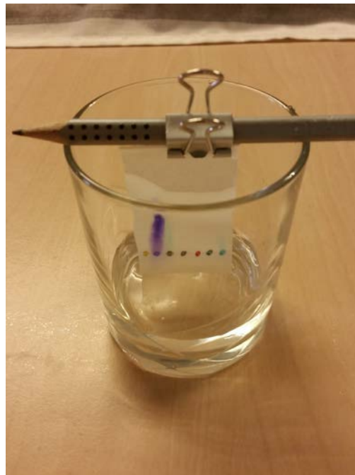
Figure 2. Paper chromatography using water as solvent. Add the solvent/water to your glass and set up the paper as described in point 5
